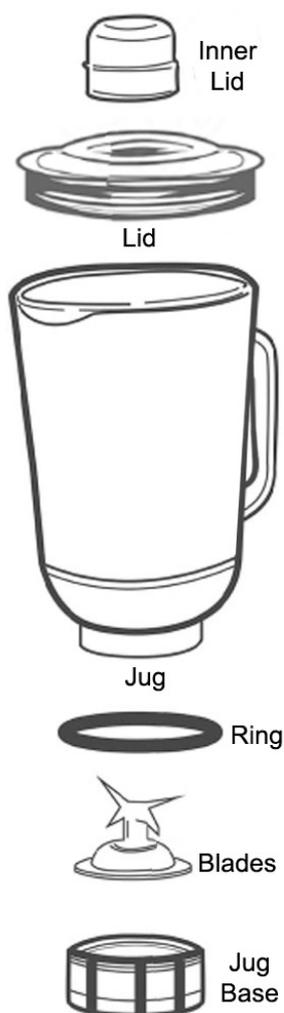
1. Put the rubber ring on the inner edge of the blades.
