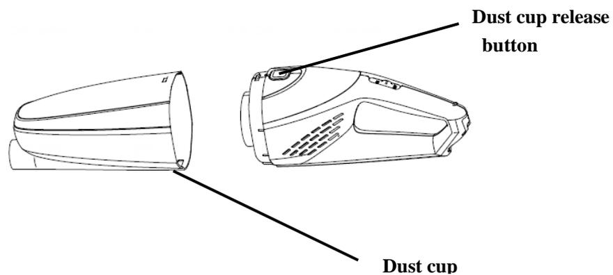
2. Grasp filter from the center. Pull filter out of dust cup then empty the tank into waste basket.
